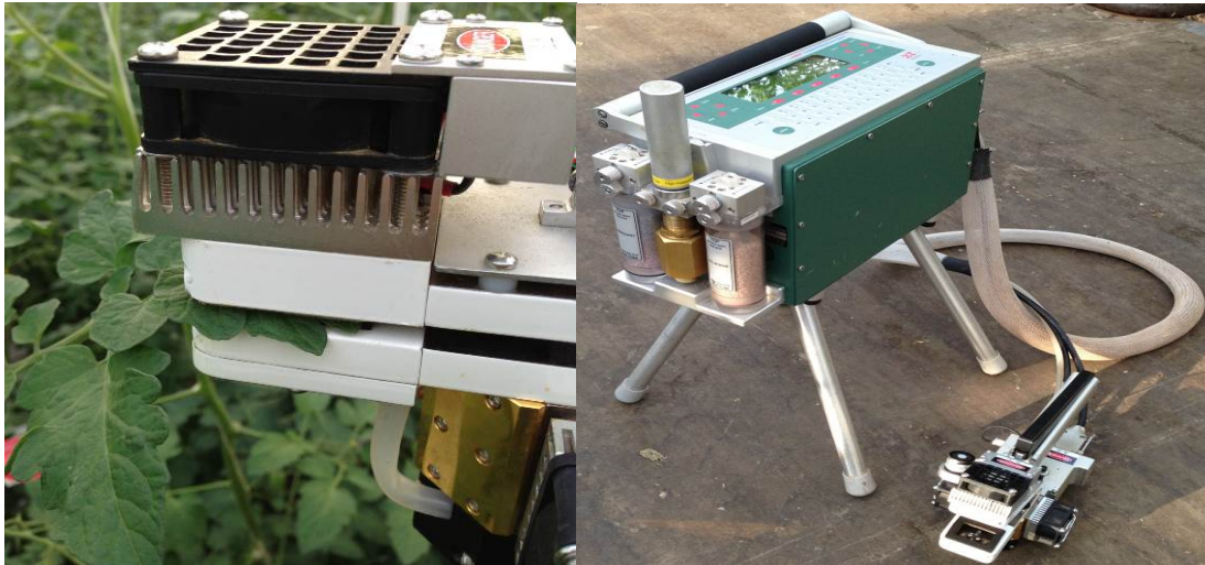
Figure i. Terminal leaflet gas exchange measurement on a commercial tomato cultivar, Cornerways Nursery, Norfolk.
